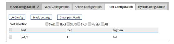
5. Enter "layer 2 configuration > VLAN configuration", check configuration result as show below.
